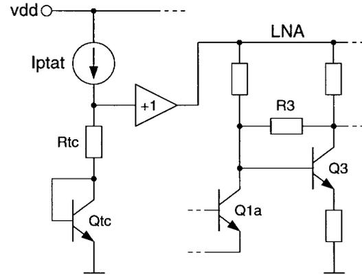
Fig. 5. Temperature compensation of LNA gain.
