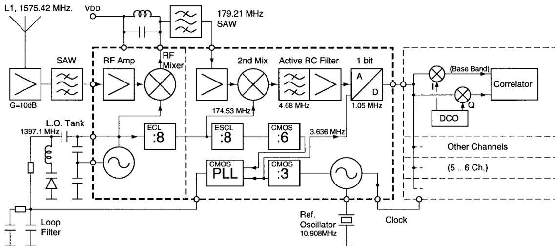
Fig. 1. Block diagram of the complete GPS receiver.
