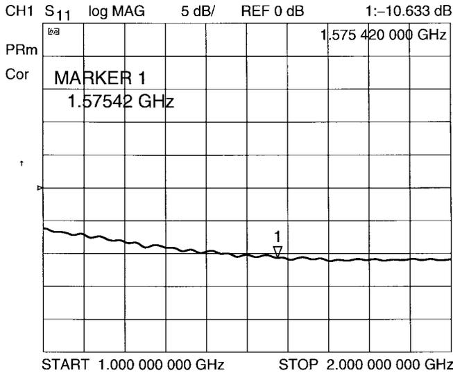
Fig. 4. Measured  $S_{11}$  of the LNA-mixer combination.
