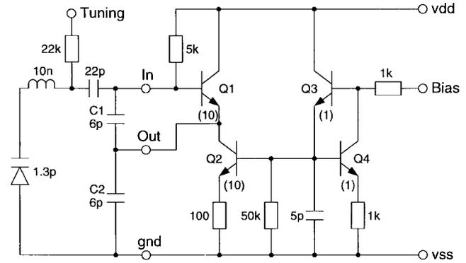
Fig. 6. Schematic diagram of the local oscillator.
