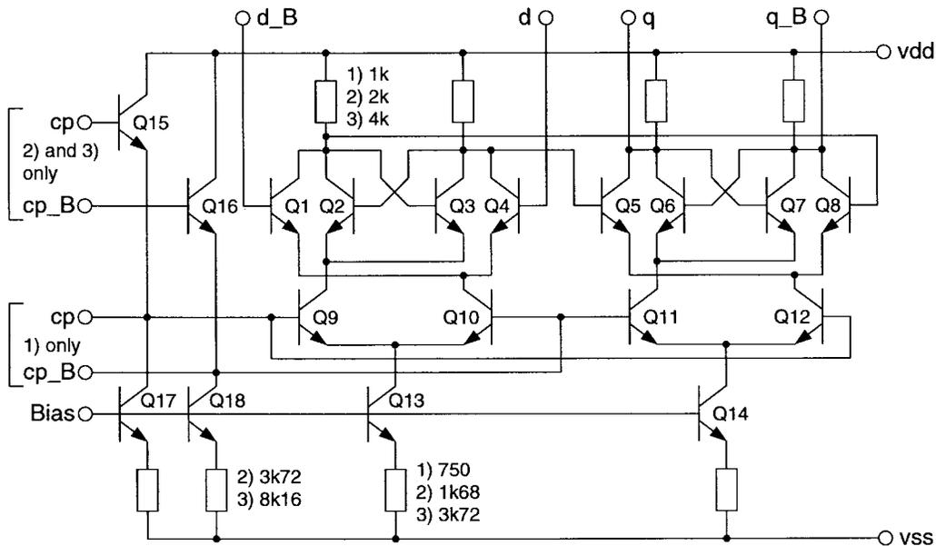
Fig. 7. Schematic diagram of the ECL prescaler.
