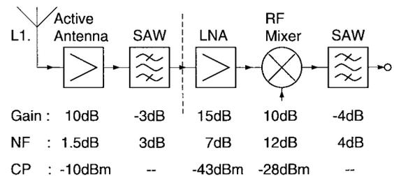
Fig. 2. GPS receiver specifications.
