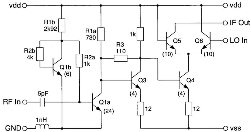
Fig. 3. Schematic diagram of the LNA-mixer combination.
