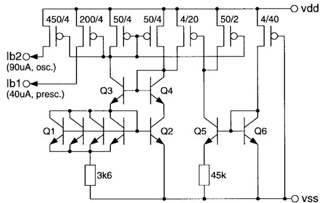
Fig. 8. Schematic diagram of the bias current source.
