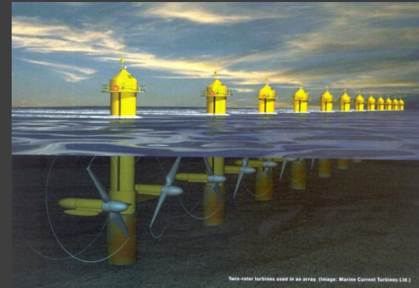
Twin-rotor turbines used in an array. (Image: Marine Current Turbines Ltd.)
